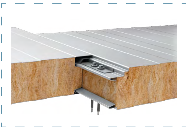
Panels connection scheme
